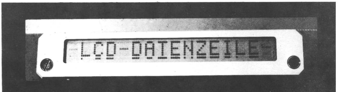
Fig. 13 Liquid crystal dot matrix display
